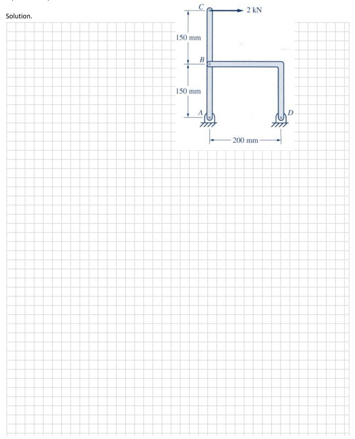
3-43 Refer to Fig. P3-43. Determine the reaction components at supports A and D due to the loads shown.
