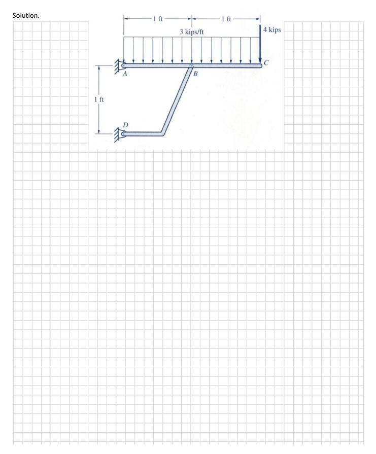
3-44 See Fig. P3-44. Determine the reaction components at the supports of the beam subjected to a uniform load as shown.
